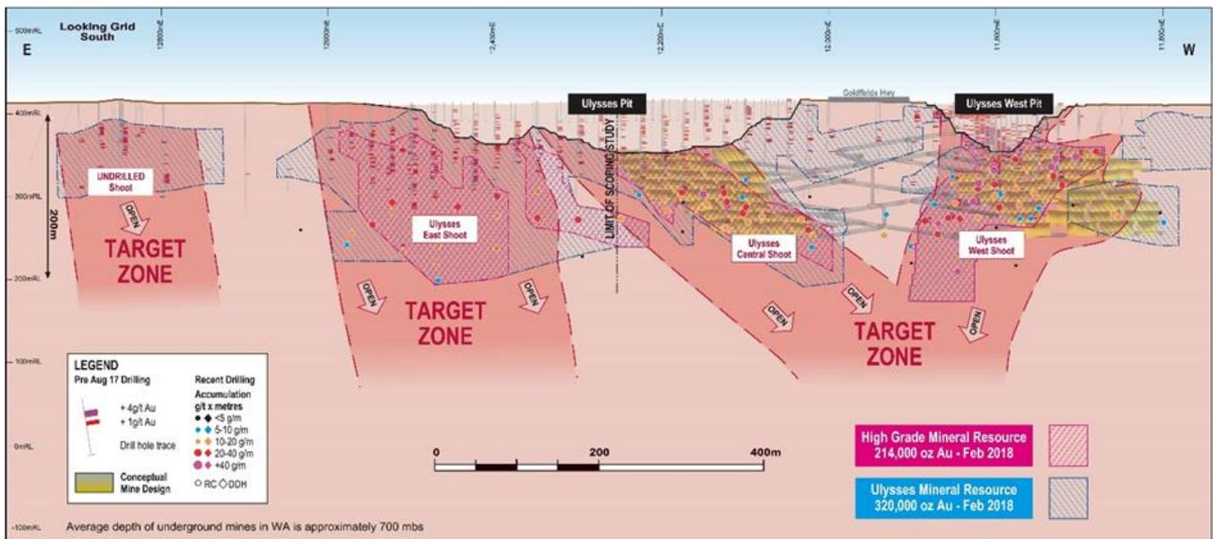
**Figure 3. Long Section in local grid showing the new Ulysses Mineral Resource (light blue outline) with the high-grade portion of the resource showing in magenta. The Resource estimate extends for over 1,500m. Note the shallow depth of drilling compared to the average depth of underground mines in WA.**
