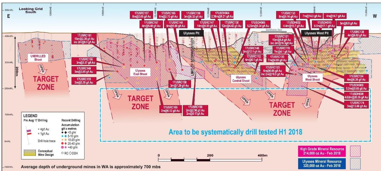
Figure 4. Long Section in local grid showing the new Ulysses Mineral Resource (blue outline) with the high-grade portion of the resource showing in magenta. Area to be systematically drill tested highlighted.
